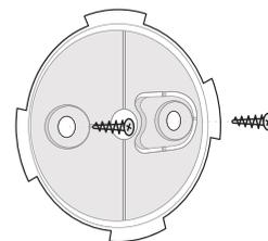
2. Put the siren on the SmartBracket panel and turn it clockwise - the light indicator will blink, confirming that the tamper has been actuated.
